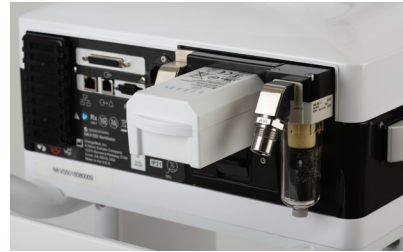
Hot swappable battery extends battery run-time.*
