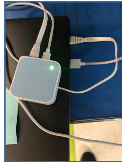
Figure 2 Connect Ethernet Cable to Access Point
