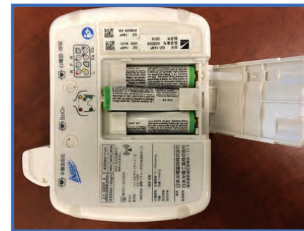
Figure 3 Install the AA Batteries into the Life Scope G3 Series GZ-140 Transmitters
