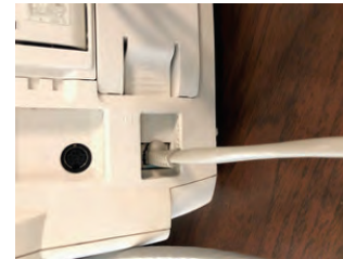
Figure 14 Ethernet Connection to Life Scope BSM-6000
